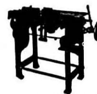
PETERS JUNIOR CARTON FOLDING AND CLOSING MACHINE. Closes 35-40 cartons per minute, no operator. Can also be made adjustable to close several carton sizes.
